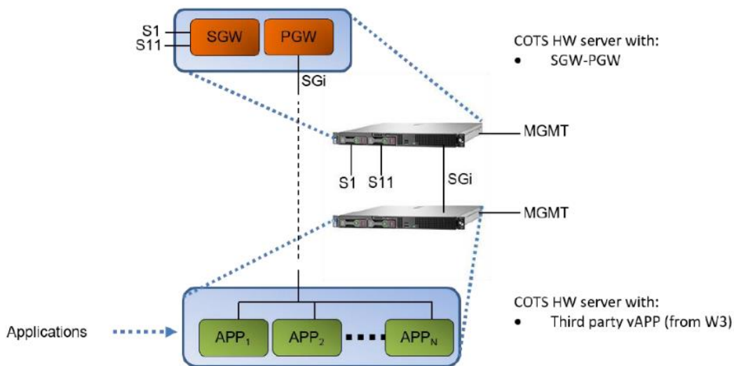
Figure 18. MEC server scheme.
