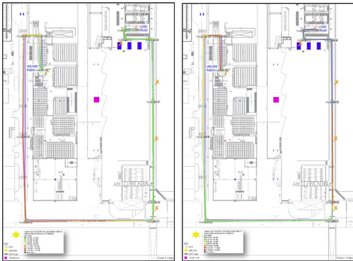
Figure 16: RSRP measurements for the indoor DOTs (Left) and the Outdoor antenna (Right) at Ford facilities
