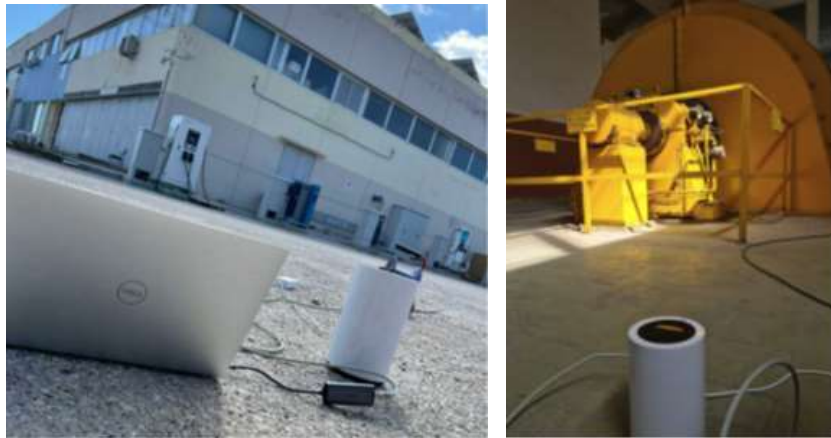
Figure 11 5G-gateway and end-user device used for network KPIs measurement.
