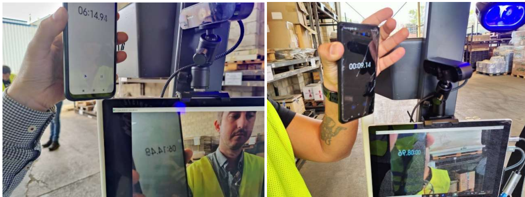
Figure 13 End-to-end video metrics for deployment on both the server and the NAO.
