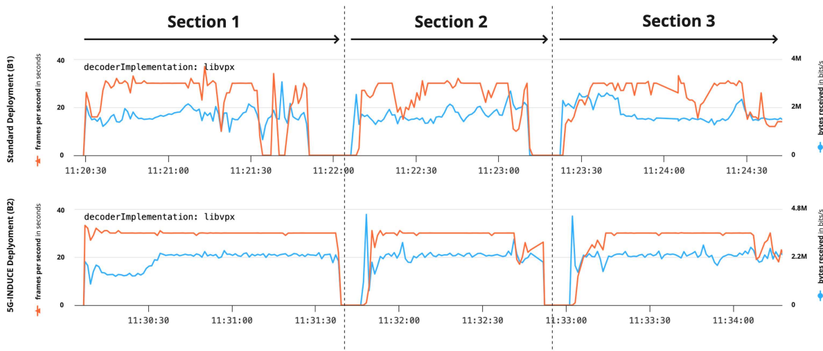
Figure 62 Measurements of bitrate and frames per second comparing deployment scenarios (B1, B2) over factory area location.
