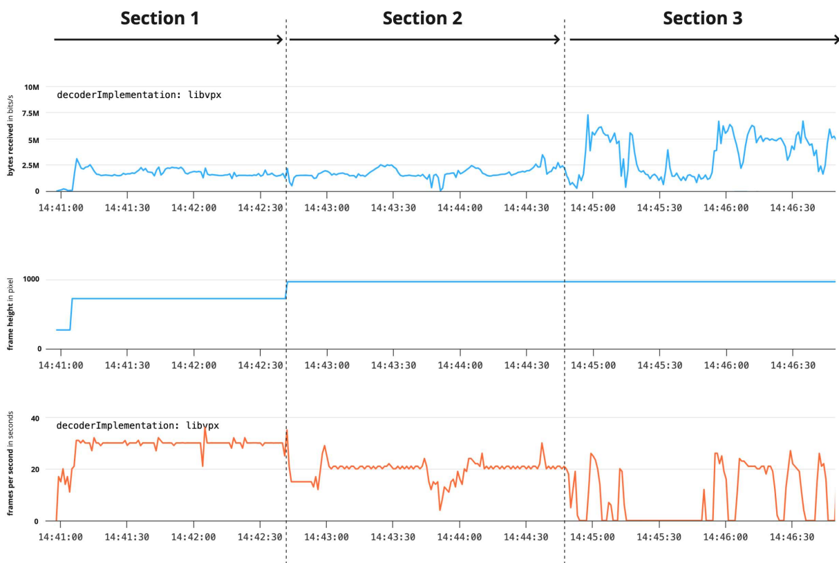
Figure 59 Measurements of bitrate, frame height and frames per second in standard MS Azure deployment (B1).
