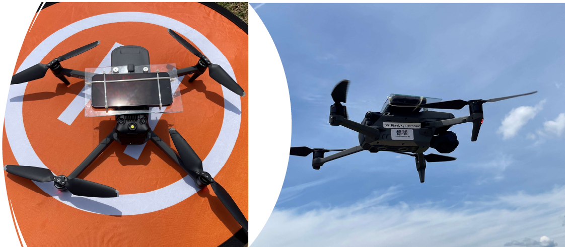
Figure 73: UC8 – Commercial Drone with Mounted 5G UE and Integrated qMON Agent.
