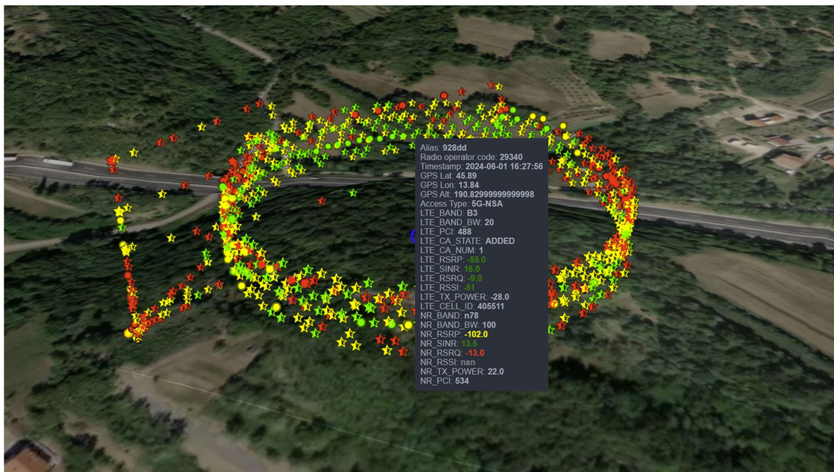
Figure 75 UC8 – Drone-based 5G NR Propagation for Operational Base Station Verification.
