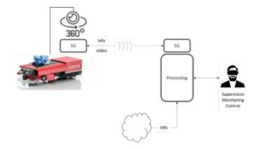
To explore VR and 5G capabilities to provide an immersive live 360 view from the AGV to a remote viewer.
