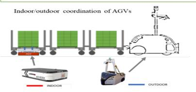
To manage a small fleet of automated guided vehicles (AGV) with simultaneous localization and mapping (SLAM) navigation, both outdoors and indoors, through 5G connectivity and edge computing capabilities.
