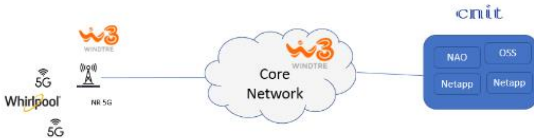
Figure 4: The physical infrastructure of the public network testbed.
