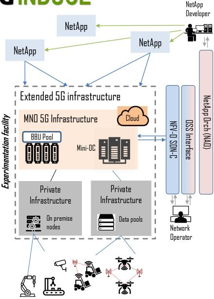
To provide an end-to-end orchestration platform over enabling experimentation infrastructures for advanced 5G NetApps applicable in the broader Industry 4.0 sector.
