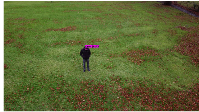
(a) Detection at 2 m with the face looking right down. (b) Detection at 7 m with the face looking right down.
