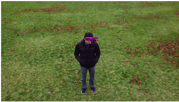
(a) Detection at 2 m with the face looking right down. (b) Detection at 7 m with the face looking right down.
