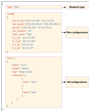
Fig. 5. A REST-API POST message example. It contains three main sections for defining the type of blueprints, TRex configuration information and VM configurations information.
